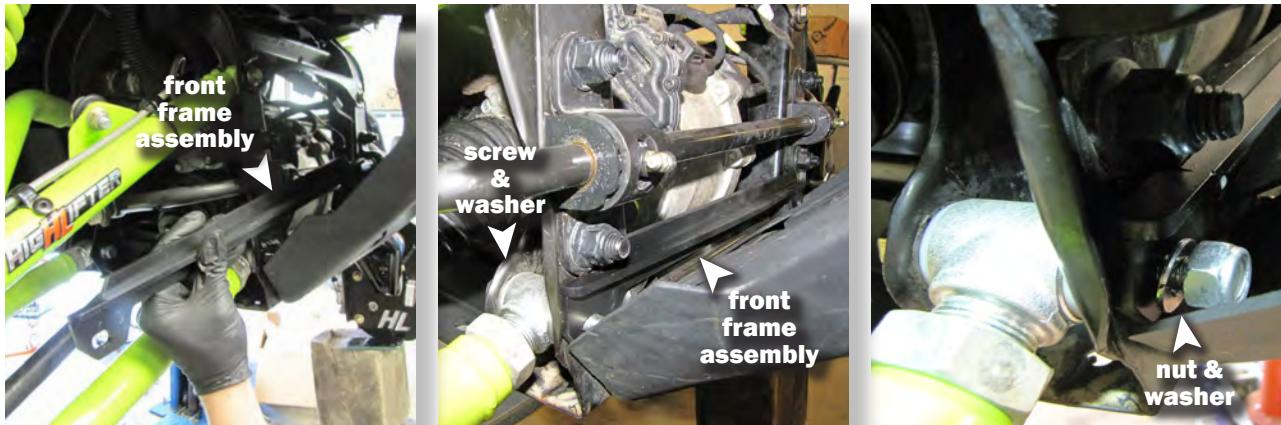
Insert Front frame assembly in front of frame, spanning the front control arms. Fasten loosely with a M10X90mm cap screw followed by a 10mm washer, secure with a 10mm washer followed by a 10mm lock nut.
