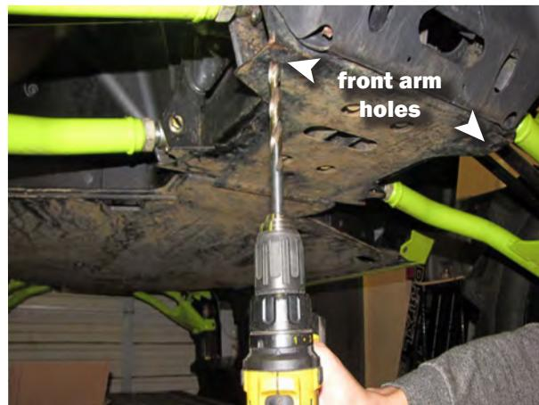
Drill out existing holes just under the front control arms with a 10mm (7/16") bit to fit M10 cap screws.
