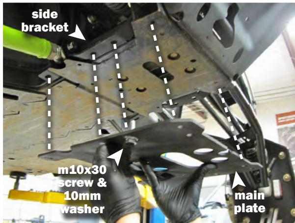
Align the main plate with the frame, rear, & side brackets. Insert one M10x30mm screw & 10mm washer into main plate & side bracket, then fasten it with a 10mm washer & lock nut to hold the plate in place while installing the remaining hardware.
