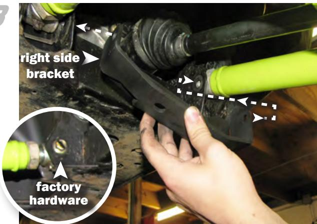
Remove the factory hardware connecting the lower control arms to the frame & align side brackets.
