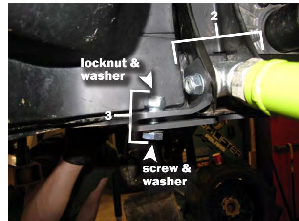
Insert M10x30mm screws & 10mm washers, into main plate & fasten with 10mm washers & lock nuts.
