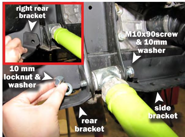
Position the rear bracket & install hardware.
